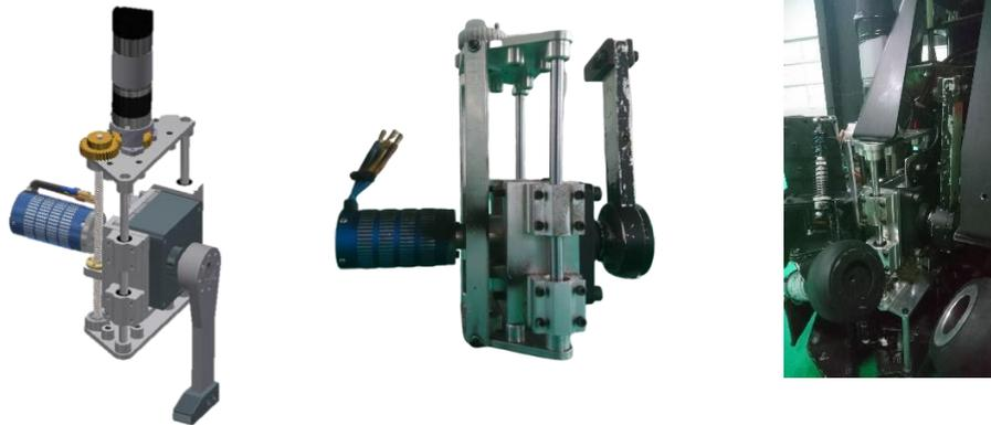
**Fig. 2.** Kicking Mechanism
