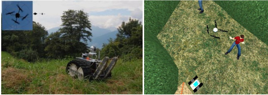
Fig. 1. Left: A Jacobs land robot cooperating with an aerial robot at the European Land Robotics Trials (ELROB) 2007 in Monte Ceneri, Switzerland. In this technology evaluation event, the aerial robot has to search for hazard areas like fire in a forest, which the land robot then has to reach. Right: A simulated RugBot and AirRobot in USARSim. Much like in the real scenario, the aerial robot will allow a much broader overview of the incident area.
