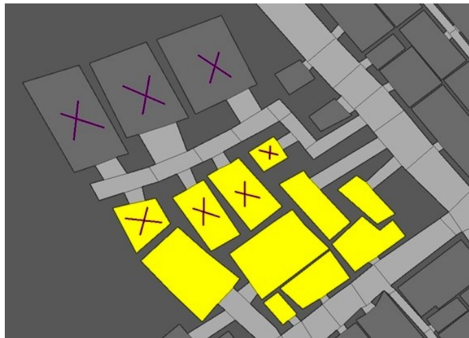
Fig 8. Zoning. Instead of the yellow buildings, buildings with purple cross should be zoned together.
