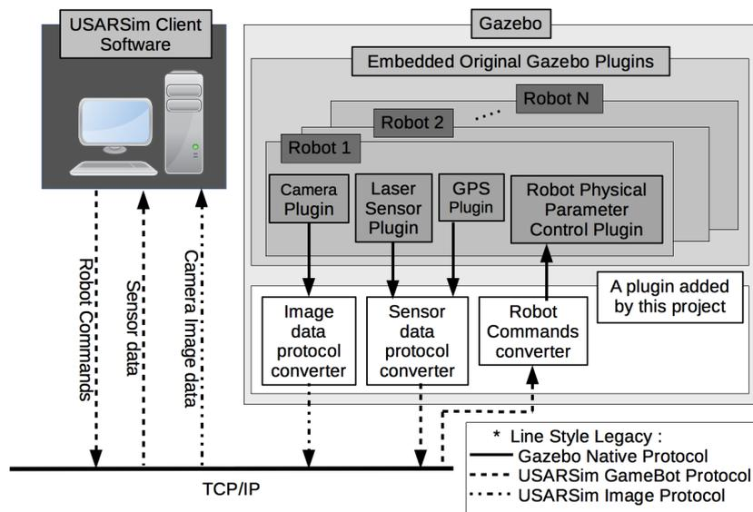
**Fig. 1.** Diagram of our prototype simulator with Gazebo. At right middle of the diagram, white blocks are our added plugin software in Gazebo. The plugin translate bidirectionally USARSim commands and Camera images and Sensor data between USARSim protocol(GameBot) and Gazebo Native protocol(Topic).
