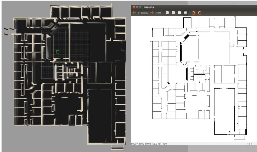
**Fig. 2.** Screenshot of 3D environment(left) and it's ground truth information(right). Ground truth information is used to calculate received Wi-Fi radio wave power strength between Wi-Fi base station and a robot or between multiple robots
