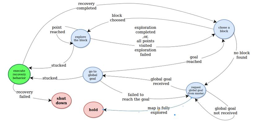
**Fig. 1.** The state machine of robot during exploration, Red color indicates a final outcome, Blue indicates a state, and Green indicates another state machine.
