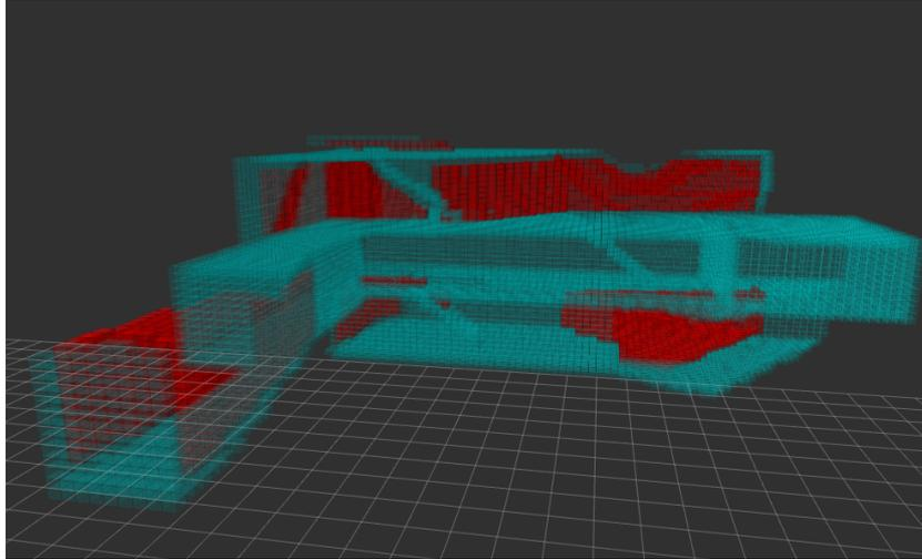
**Fig. 4.** Detected frontier cells (red cells)
