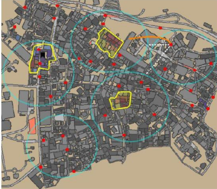
Fig.2: Select fire clusters by fire brigade agents. (D1 and D2: distance from the specified agent to the fire clusters with different temperatures)
