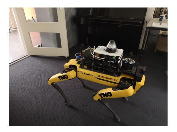
Equip the Spot robot with a DreamVU PAL camera, which gives panoramic depth images.
